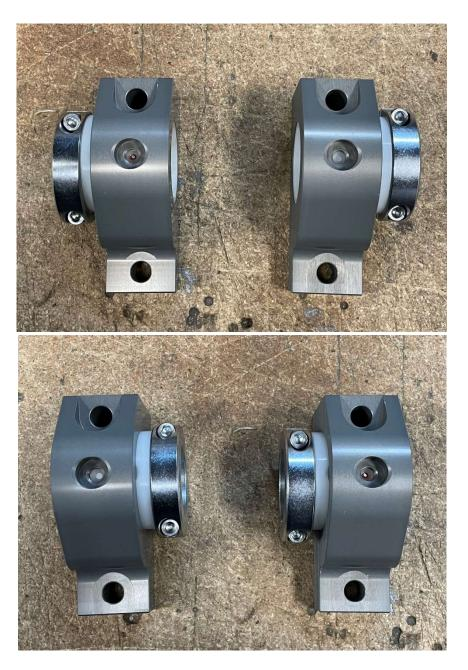
The image on the right is an example of an INCORRECT mounting process. The bar will be retained from moving side to side as the clamps will rub on the mounts (this will likely wear and make noise!) however the bushings will likely wiggle their way out of the mounts, again as the grease zerks are not designed to hold the bushings in place.
