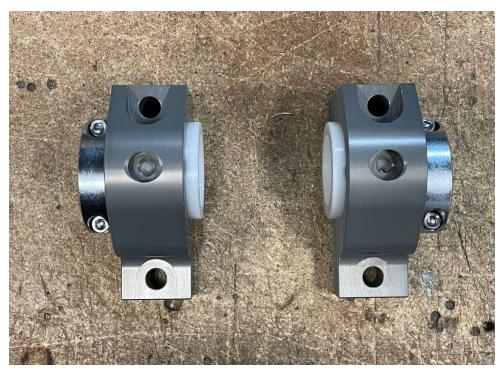
IF the bushings are not inserted so that the flanges are opposite each other, then that will need to be addressed first by disassembling the SwayLOC from the torsion bars and reassembling with the bushing in one of the approved designs listed above.
