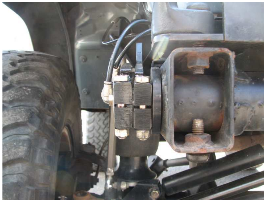
Figure 7 Finished install, note the gap between the inner and outer arms.
