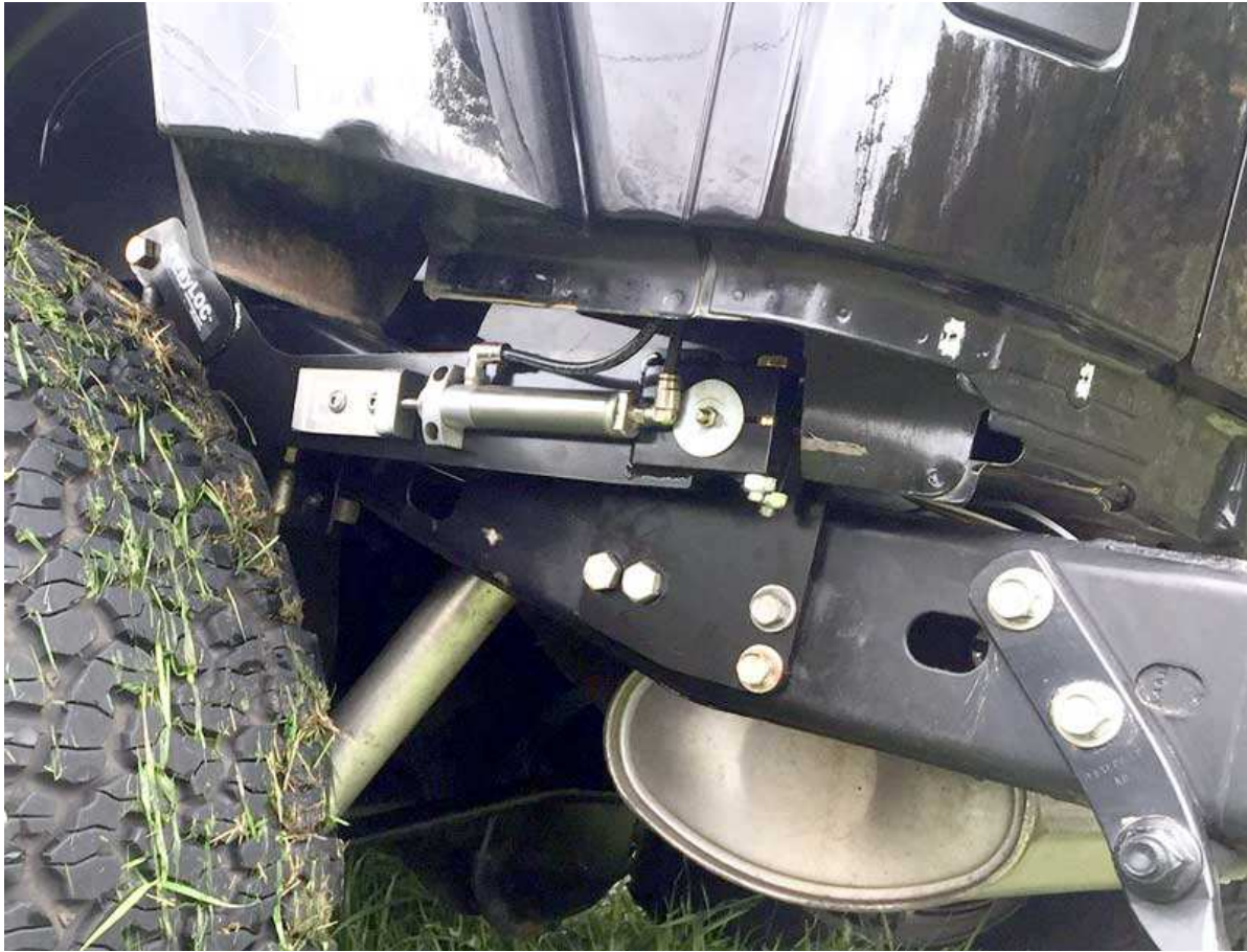
JK Rear SwayLOC installed
