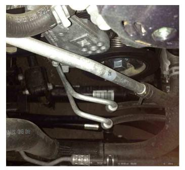
Now, grab the york. Position it so that the ORO Clutch Drive Couple is away from you, and carefully lower the york assembly down towards the harmonic balancer. You may find it easiest to position the york just forward of the passenger side valve cover, and lower it down from there. You can set it on the cross member, along the power steering return line, if you need to release and adjust your grip
