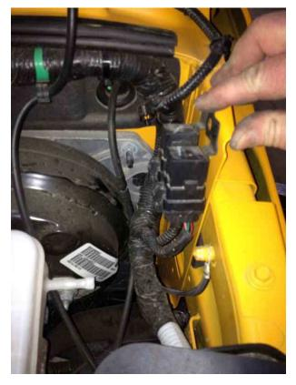
With the relays removed, you will drill 2 holes, 3/16" diameter, in the inner fender to mount the bracket. The first hole, positioned as shown in the image to the right, will be drilled 3/4" rear of the forward edge of the raised inner fender structure. The hole should be approximately 1/4" down from the doubling panel as shown. This hole will align with the hole drilled in the bracket. You will need to drill a second hole to line up with the lower slot of the bracket.
