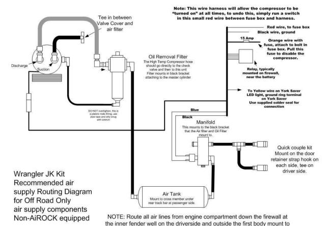
The 3/8" airline goes out of the coalescing filter to the air tank, routed down the fender, outside the front body mount, along the framerail, tucked under the rockrail tabs and tucked along the top of the framerail to the fuel filler line, and to the tank.
