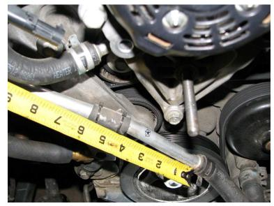
Next, Locate the longer single aluminum spacer. There is only 1 that will fit over the 10mm stud that you installed 2 steps ago. Slip the spacer over the stud and slide it up to the engine mount.
