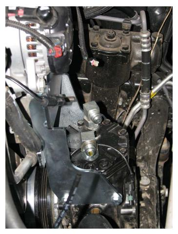
Now it is time for the lower bracket. This one installs to the bottom surface of the oil pan and mounts to the 2 rearward lower mounting holes on the york itself.
