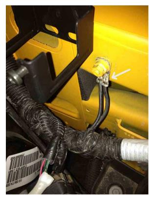
Now its time to mount the air supply bracket, the bracket that holds the manifold and the AiROCK Control Unit (ACU) This bracket mounts to the inner mounting bolt of the master cylinder and will mount to the inner fender with 2 self tapping screws in holes that you will drill. On the right is the bracket, in position. .
