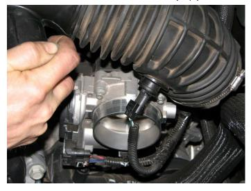
The air cleaner is held in place by 3 plastic pins that are secured into rubber cups on inner fender. Grab hold of air box and give a sharp upward tug to remove air box. Set the air box off to the side.
