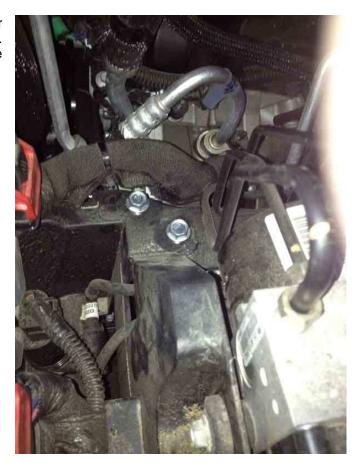
With the mounting bracket in place, mount the manifold to the bracket. There is 2 threaded holes in the back of the manifold that mount it to drilled holes in the bracket. Use the  $10-24 \times \frac{1}{2}$  screws to mount it.
