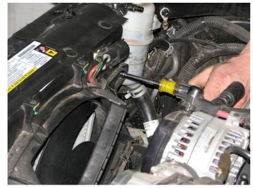
Once these 2 screws are removed, simply remove the cooling fan and shroud assembly. We've found that working the driver side up first and removing it at an angle as shown in this image to be the easiest way. You'll need to wiggle the fan shroud to get the retaining bolt area to clear the upper radiator hose and then should be able to lift it out.
