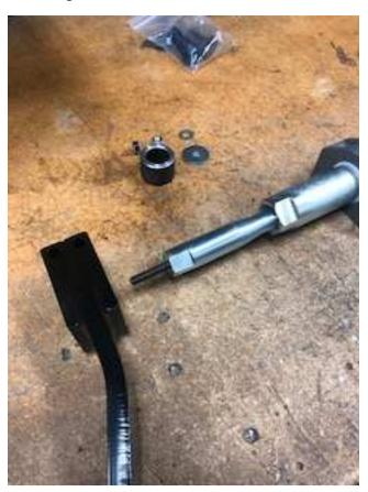
Place the arm over the stud, install the large heavy washer, the small washer and a 5/16" nut on the stud. Rotate the bar to match the keying of the hub and snug the nut by hand. Then using a  $\frac{1}{2}$ ' wrench, start tightening the nut. MAKE SURE that the arm/hub assembly stays perpendicular to the torsion bar, the RED and YELLOW stripes need to stay perpendicular. Failure to do so may result in the bar digging into the hub. The fit is designed to be snug.
