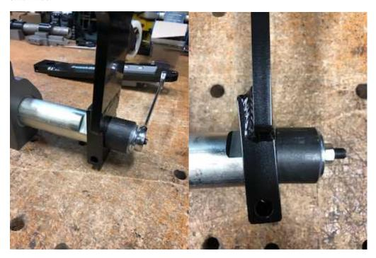
Again, using the sleeve, washers and nut, as you tighten the  $\frac{1}{2}$ " nut the hub should slide over the outer bar. MAKE Sure that the hub is perpendicular to the bar, as this one will try to go on at an angle like shown, we find that you can usually hold the rearward edge just enough to get it to go on straight. Sometimes a small tap from a hammer will right itself.
