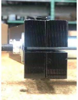
Once you have the bar fully seated, install the 3/8" cross bolt and the locking nut (the nut is installed with the wider face towards the hub!) and torque the nut to 50 ft lbs. Place a large washer and the 5/16" x  $\frac{1}{2}$ " bolt onto the endo of the torsion bar and tighten as well. Please note, you NEED to tighten the clamp bolt as the end cap bolt will not hold the hub on when doing the next process.
