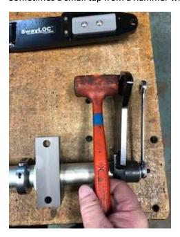
By now, you probably have the feel of, the last arm, the latching arm, is by far the easiest. SRemember to open the latch by flipping the level to the rear or is a remote version, slide the latch open and using one of the  $\frac{1}{2}$  jam nuts, jam the latch open for the next step.
