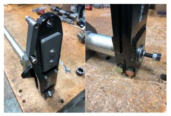
Once you get the arm fully seated, install the 3/8" clamping bolts, torque to 50 ft lbs, and then remove the stud. We include a second nut in case you need to double nut and lock them together to get a wrench to remove the stud.
