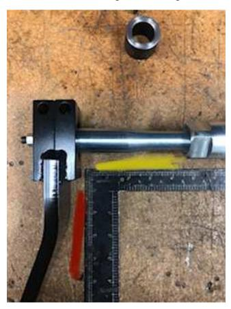
Once you can tell that the bar is sliding into the hub, keep tightening the nut until the bar stops sliding. It should be nearly flush with the outside of the hub, or just a hair short.
