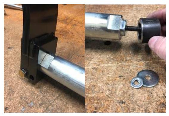
Now, with the install tool assembled as shown, when you tighten the nut, this will drive the outer bar into the dual hub side. AS you start to tighten it, rotate the bar slightly, make sure that the outer bar is rotated and aligned with the hub interfaces, again, if you force it without it being aligned property it may scar the opening and you will likely have to fill the burr out to get it to assemble.
