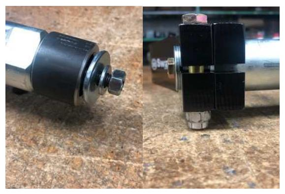
Now, simply tighten the nut and the outer bar should slide into the hub on the dual hub side. Make sure to check that it fully seats itself before you stop tightening the nut the outer bar should be able to be seen butting up the side of the small hub thru the gap in the slot. Note the 3/8" bolt and lock nut arrangement for the small hub. Insert the 3/8" bolt in the large hub, tighten to 50 ft lbs.
