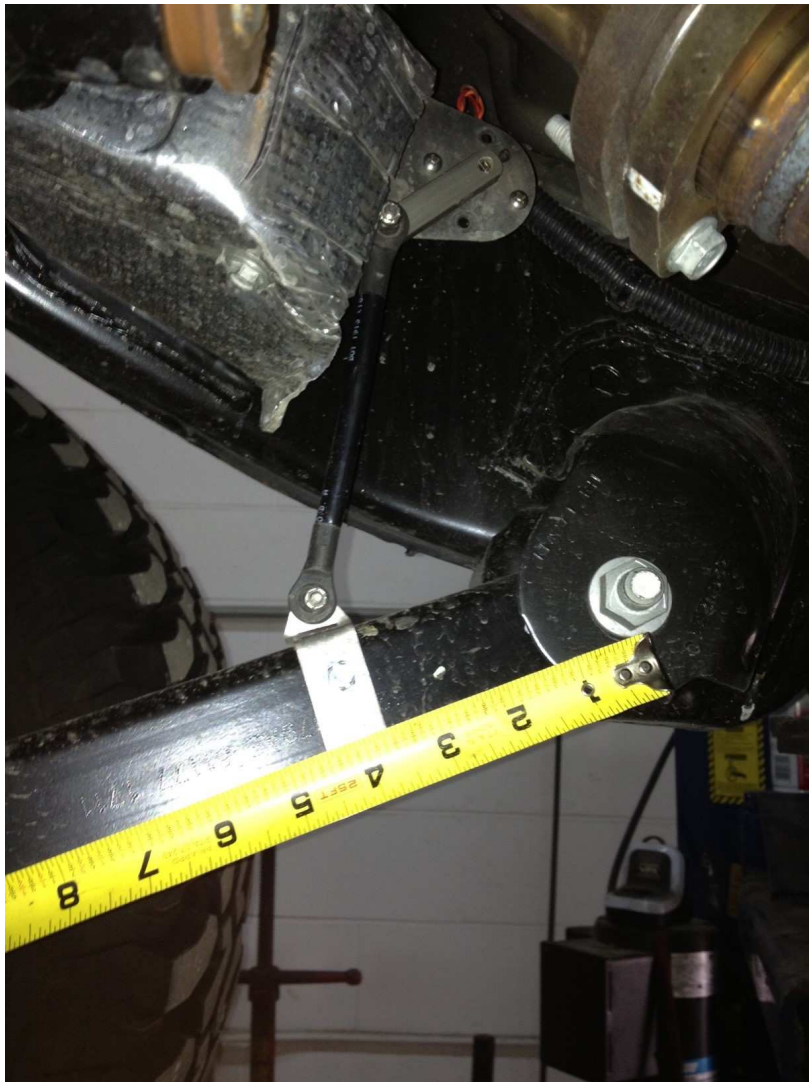
Right front height sensor (H2 Green) installed.
