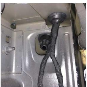
11. To connect to the taillight circuit for the license plate light, the easiest way is at the taillight electrical connector.
