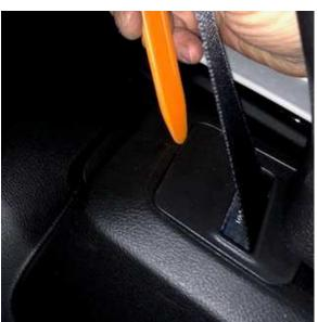
Once the ring is disconnected, you should be able to wiggle the subwoofer enclosure free and turn the rear edge towards the driver side. It should pivot at the forward edge of the enclosure and stay as shown in this image.
