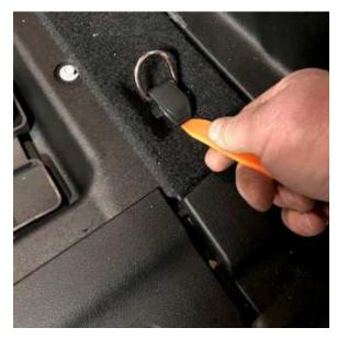
4. Remove right side floor panel and set it off to the side. At this time, also remove the little tool tray from the rear edge, between the tailgate and the underdeck compartment. Set if off to the side as well.
