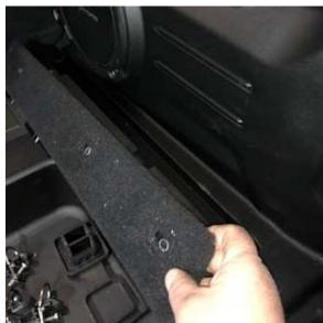
5. Remove the rubber seal from the vertical and right side along the lower edge, just slide it away from the subwoofer panel so it can be reinstalled after the subwoofer goes back in.
