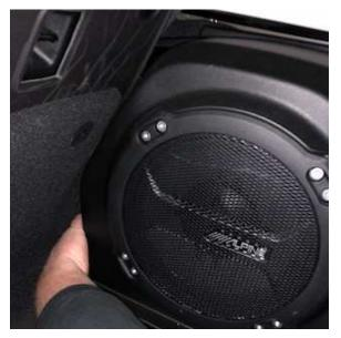
7. With a trim tool or a screwdriver, lift the forward edge of the seat belt trim ring, to unclip it from both the subwoofer enclosure as well as the enclosure that stays between the roll bar and the window. With the subwoofer popped free as in step 6 above, simply grab with your fingers and lift the tabs free.
