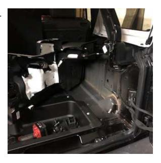
9. On top of the plastic panel that has a small cover, this small cover gets access to the 1 retaining bolt for the tail light. Gently lift the cover, there is a small opening on the window side that you can use a small screw driver to release the tab then lift this cover out of the way.
