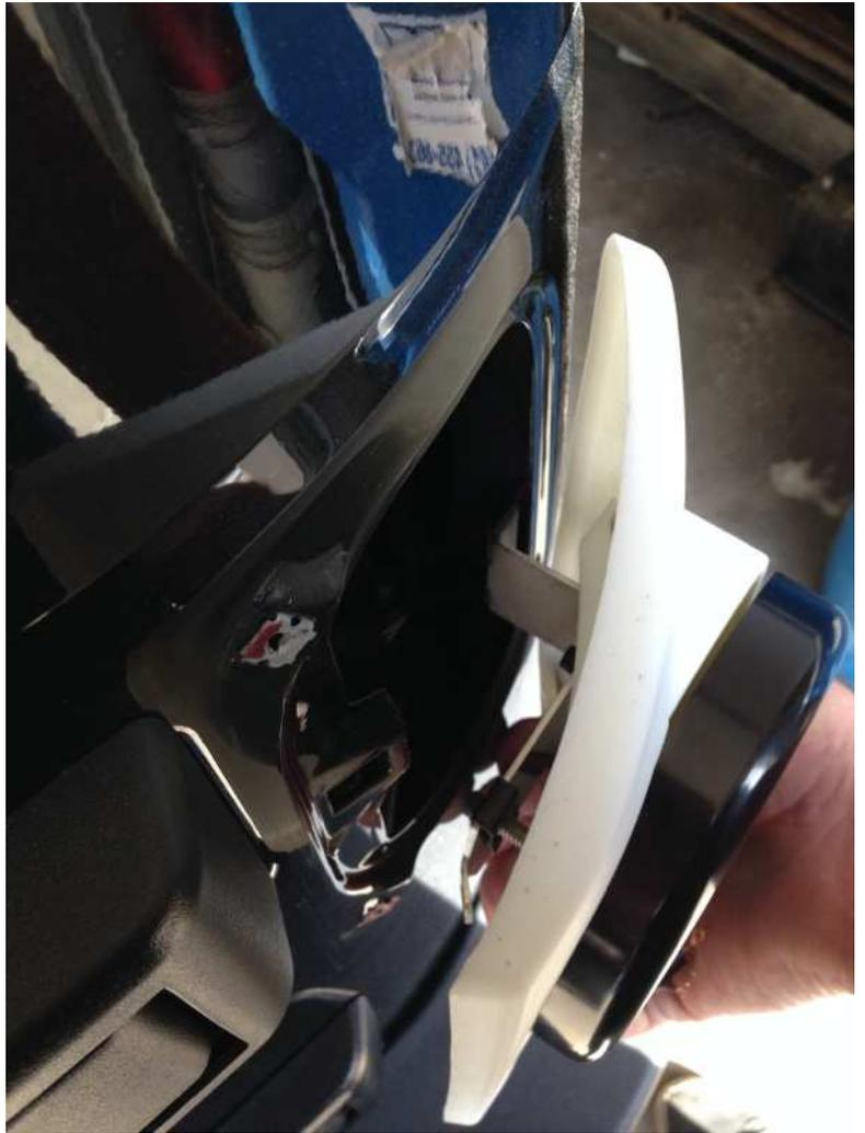
At this point, the tailgate side of the stainless bracket should be able to clear the opening as you push the assembly towards the Jeep. Once it gets behind the sheet metal, raise the assembly into the proper position, the top of the LitePANEL should be about 1/8" below the body line when positioned properly.
