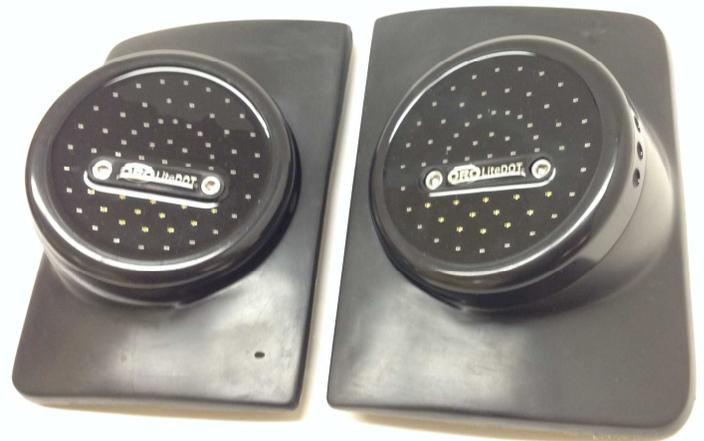
The wires going into the back of the LiteDOT will be below the 2 mounting bolts. You will determine the left or right panel by placing the left or right LiteDOT upon the panel, and when correct the holes for the mounting bolts and wires will line up.
