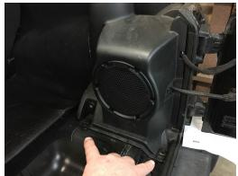
The plastic tailgate guard along the tailgate is removed by lifting gently along the bottom edge. The spring clips (5 of them) will release and the cover rotates with the bottom coming away from the tailgate, the top stays clipped in until the bottom is fully released.
