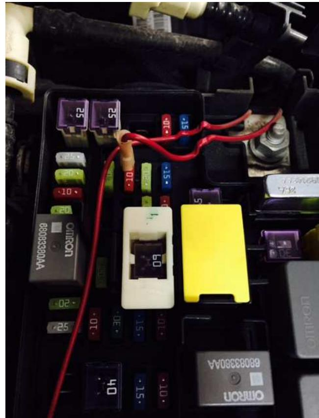
The last wire is the gray wire. This the one that needs to be tied to the positive side of the dome light circuit. Some JK's have a small LED light in the foot well, you can dissect this light and tie into the power side of this circuit. If your Jeep doesn't have this factory foot well lighting, you will need to remove the instrument cluster to find the dome light control circuit to tie this gray wire to.
