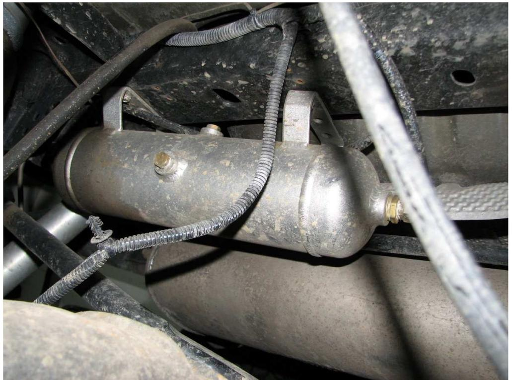
On the wiring harness, route the wires safely so as to not get caught in the engine. There is a wire with a weatherpack connector on it coming off the relay. This attaches to the York Compressor.
