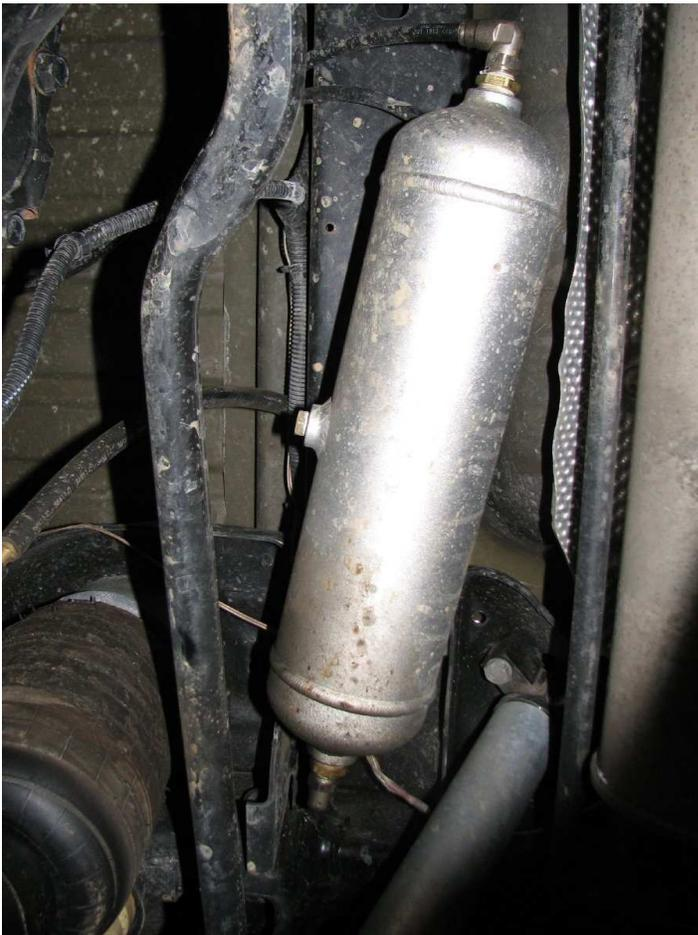
Mount the air tank to the crossmember that runs above the rear track bar, as seen in the image to the right. Run 3/8" airline from the tank back to the manifold. The Manifold is designed to be bolted vertically to the driver's side of the filter bracket, with one port on top and 2 ports will face to the driver's side of the vehicle. The top port goes to the
