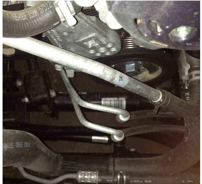
Now, grab the yolk. Position it so that the ORO Clutch Drive Couple is away from you, and carefully lower the yolk assembly down towards the harmonic balancer. You may find it easiest to position the yolk just forward of the passenger side valve cover, and lower it down from there. You can set it on the cross member, along the power steering return line, if you need to release and adjust your grip
