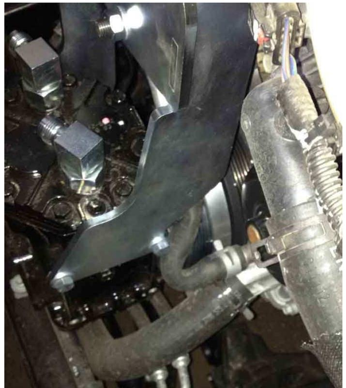
The rubber hose with the brass fitting on one end and the plastic tee on the other is the air inlet. The brass fitting goes to the compressor fitting that attaches to the compressor port marked "suction", on the driver's side when using our yolk.
