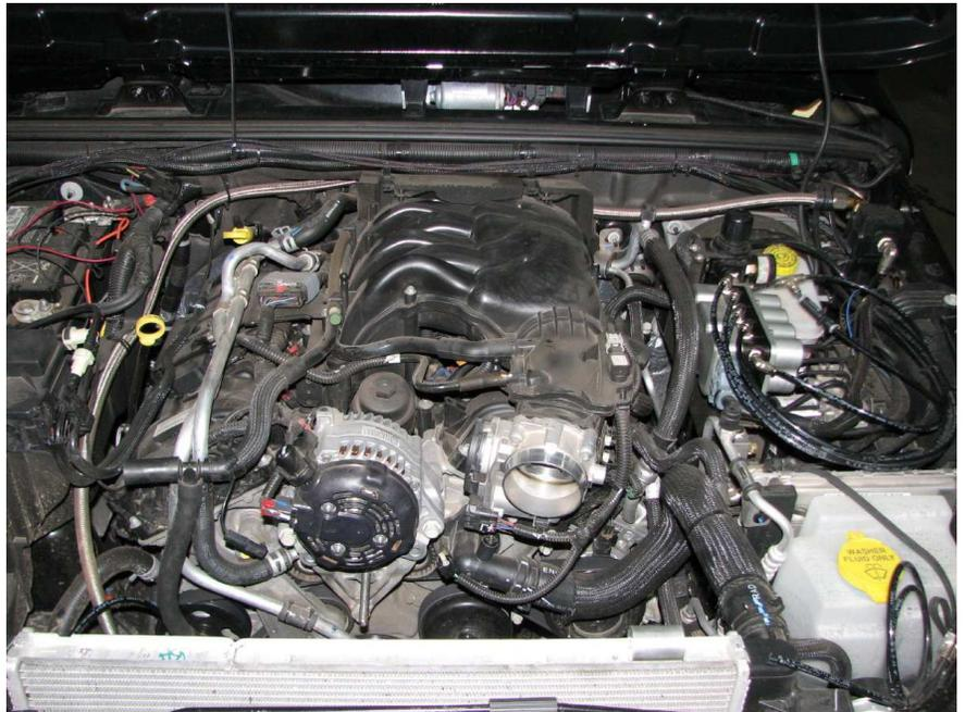
Once the compressor is mounted, you need to inspect the coolant return line that you attached the rubber hose to earlier. This line will be held rearward by the bracket against that rubber hose you ziptied over it earlier. This rearward pressure, on some models, results in the rubber hose at the lower end where it attaches to the engine to possibly kink in 2 locations. These locations are highlighted by arrows in the image to the right.
